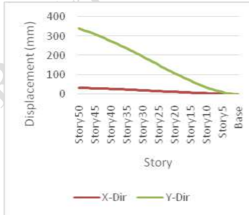
Fig 4.2- Displacement in Y-axis
